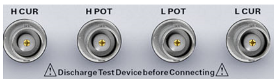
Fig. 8.1: Front panel BNC connectors
