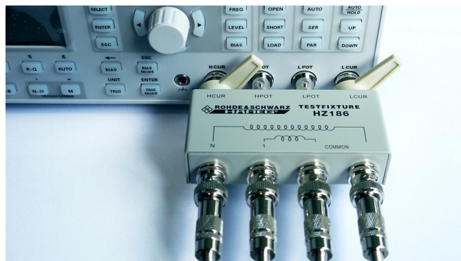
Fig. 8.6: Connecting the measurement adapter to the LCR bridge
